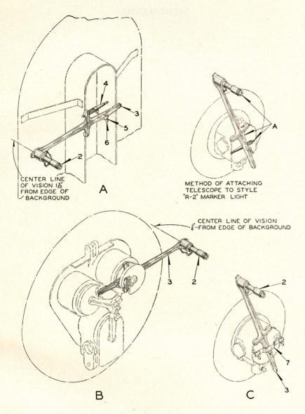
Sighting Telescope With Mounting Fittings for Aligning Styles "L", "P-2", "R-2" and "TR-2" Color Light Signals and Styles "R-2" and "HC-33" Marker Lights
