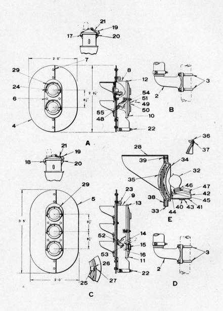
TWO AND THREE-COLOR STYLE "N" LIGHT SIGNAL UNITS AND MOUNTING FITTINGS
