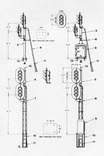
2-UNIT, TWO AND THREE-COLOR STYLE "N" LIGHT GROUND SIGNALS, COMPLETE WITH POSTS AND MOUNTING FITTINGS
