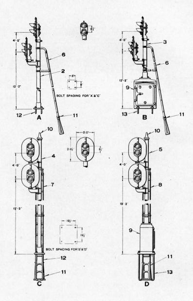
2-UNIT, TWO-COLOR STYLE "N" LIGHT GROUND SIGNAL, COMPLETE WITH POST AND MOUNTING FITTINGS
