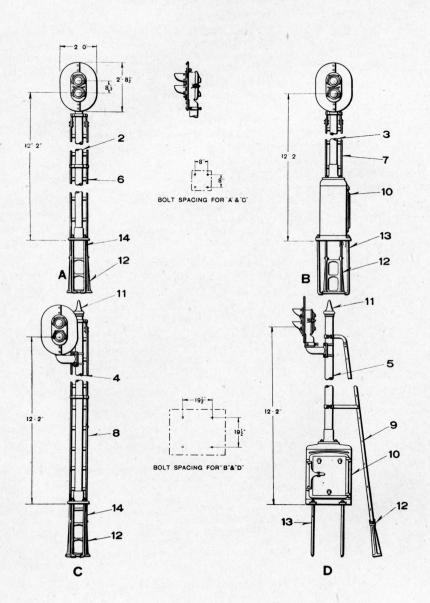
1-UNIT, TWO-COLOR STYLE "N" LIGHT GROUND SIGNAL, COMPLETE WITH POST AND MOUNTING FITTINGS
