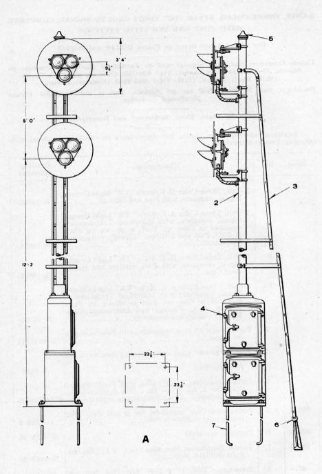
2-UNIT, THREE-COLOR STYLE "TR" LIGHT GROUND SIGNAL, COMPLETE WITH POST, DOUBLE INSTRUMENT CASE AND FITTINGS
