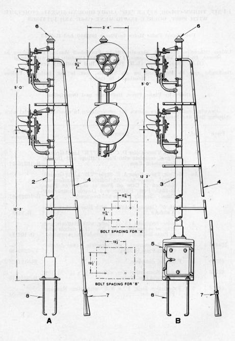
2-UNIT, THREE-COLOR STYLE "TR" LIGHT GROUND SIGNAL, COMPLETE WITH POST AND FITTINGS
