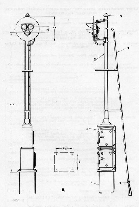
1-UNIT, THREE-COLOR STYLE "TR" LIGHT GROUND SIGNAL, COMPLETE WITH POST, DOUBLE INSTRUMENT CASE AND FITTINGS
