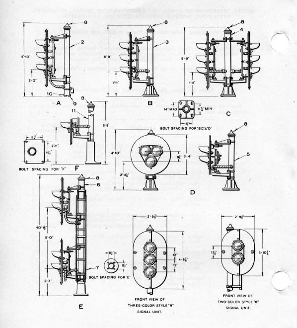
1 AND 2-UNIT, TWO AND THREE-COLOR STYLE "R" AND "TR" LIGHT BRIDGE AND BRACKET POST SIGNALS, COMPLETE WITH POSTS AND FITTINGS
