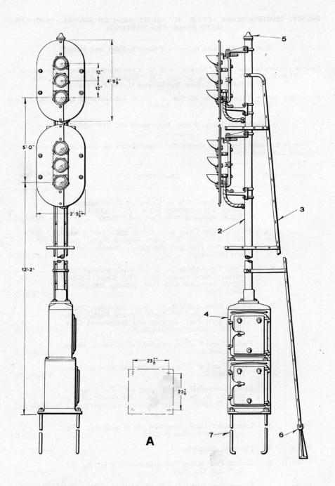
2-UNIT, THREE-COLOR STYLE "R" LIGHT GROUND SIGNAL, COMPLETE WITH POST, DOUBLE INSTRUMENT CASE AND FITTINGS
