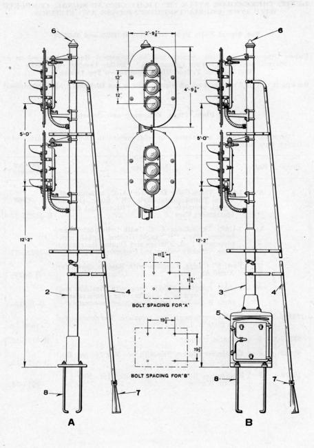
2-UNIT, THREE-COLOR STYLE "R" LIGHT GROUND SIGNAL, COMPLETE WITH POST AND FITTINGS
