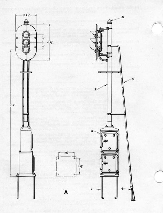
1-UNIT, THREE-COLOR STYLE "R" LIGHT GROUND SIGNAL, COMPLETE WITH POST, DOUBLE INSTRUMENT CASE AND FITTINGS
