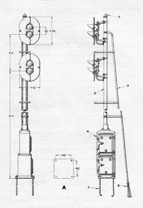
2-UNIT, TWO-COLOR STYLE "R" LIGHT GROUND SIGNAL, COMPLETE WITH POST, DOUBLE INSTRUMENT CASE AND FITTINGS
