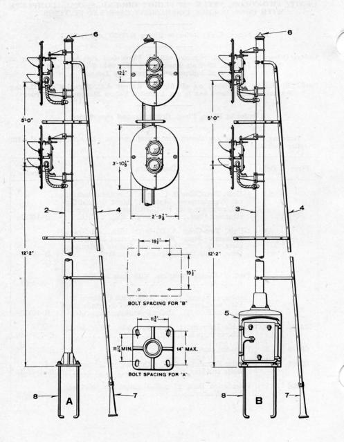
2-UNIT, TWO-COLOR STYLE "R" LIGHT GROUND SIGNAL, COMPLETE WITH POST AND FITTINGS
