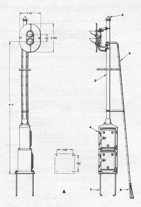
1-UNIT, TWO-COLOR STYLE "R" LIGHT GROUND SIGNAL, COMPLETE WITH POST, DOUBLE INSTRUMENT CASE AND FITTINGS
