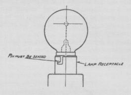
In replacing incandescent lamps, lamp base must not bind in lamp receptacle sufficiently to prevent spring in base of the receptacle from forcing pins in lamp base to their proper seats. This is necessary in order to have the filament in its correct location.
