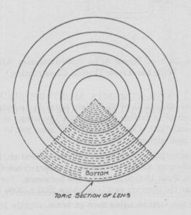
examined to see that the lens is in its proper position. The lower portion is indicated by the word "bottom" imprinted in the glass and under no circumstances should this be turned to any other position. This is true of both the ordinary toric and the spreadlite toric.
