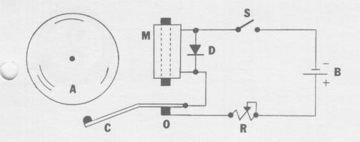
Figure 2 is a schematic diagram of the operating parts and circuit for a highway crossing bell.
